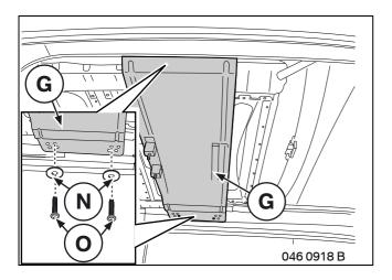
Adhere fleece band **G** to retaining plate (1) of DVD console **D** (cut off excess length).
