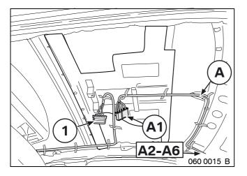
Secure branch **A1** in roof with insulating tape. Route branch **A2-A6** along the main wiring harness down to the right-hand D-pillar.
