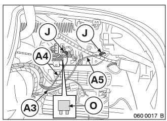
Connect branch **A3** to battery terminal **B+**. Plug branch **A4** into 32-pin black connector **X11012**, **PIN 16** or connect to GN/BL wire with insulation displacement connector **J**.
