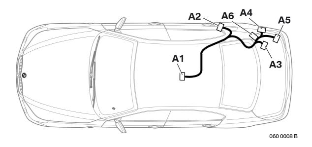
Install all wiring harnesses as illustrated and secure with cable ties. Tie back excess length.
