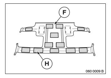
Adhere damping strips **H** to top of roof brace **F**.
