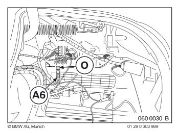
Fit fuse **O** (3A) in branch **A6** and tie back to wiring harness.
