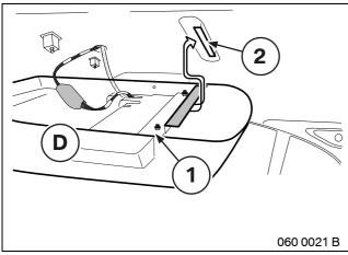
Take particular care when mounting the DVD console to ensure that the connection cables are not trapped or damaged. ◀
