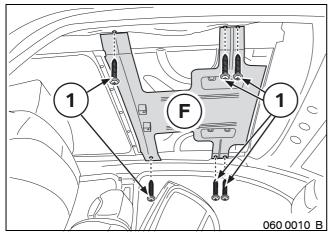
Secure roof brace  ${\bf F}$  with screws (1) for sliding sunroof cassette.
