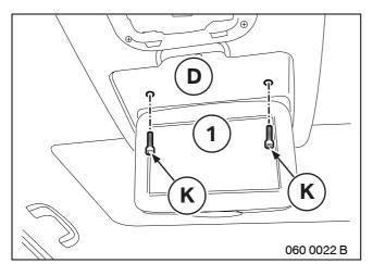
Fold down monitor (1) . Firmly secure DVD console  ${\bf D}$  with two screws  ${\bf K}$  to the roof brace.
