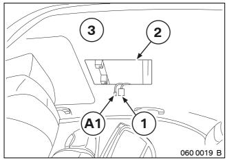
Pass branch **A1** and interior lighting connector (1) through opening (2) in headlining (3).
